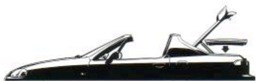
Place roof in its hinged holder frame
